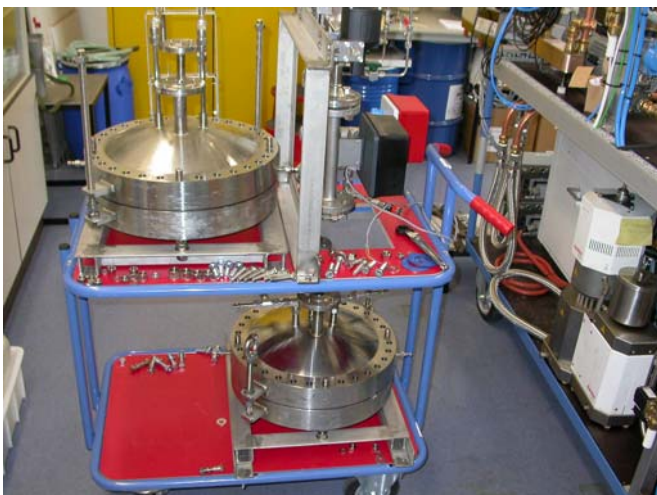
Figure 4: Test installation for a thermo chemical heat pump
