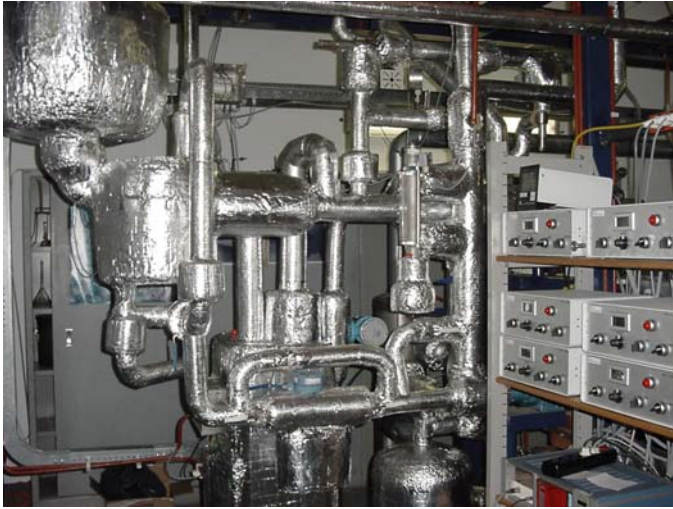
Figure 5: Test installation for a compression resorption heat pump
