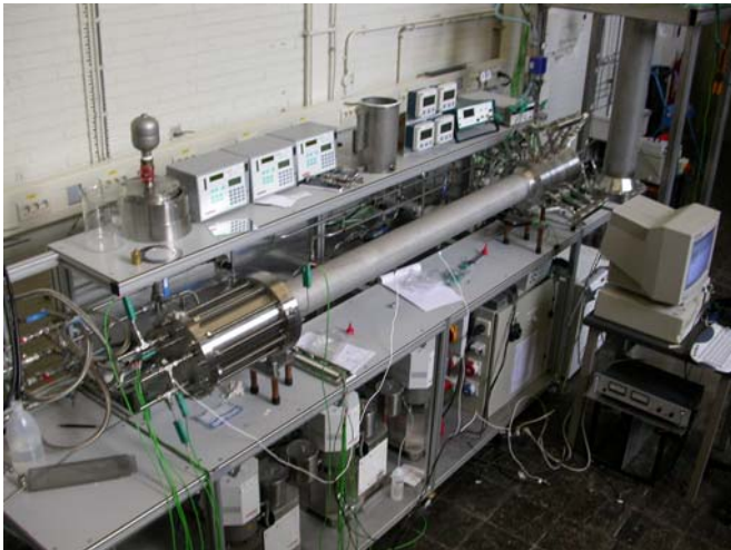
Figure 3: Test installation for a thermo acoustic heat pump
