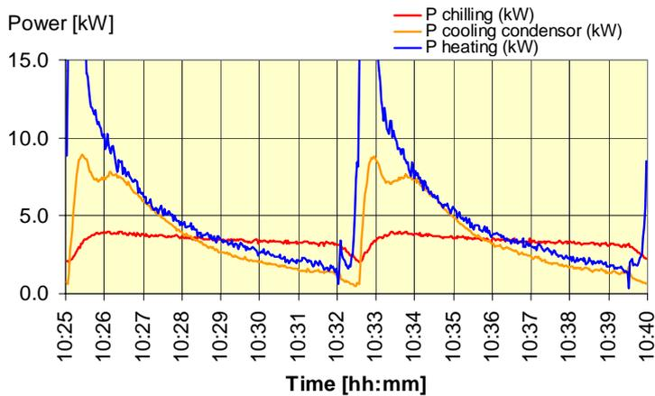
Figure 3.2 *Thermal power for heating the sorbent reactor, cooling of the condenser and chilling of the evaporator during the 15-minute cycle under standard conditions*
