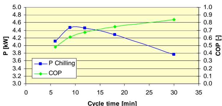
Figure 3.1 Chilling power and COP as a function of cycle time at inlet temperatures:  $T_{heating} 85^{\circ}C$ ,  $T_{cooling} 25^{\circ}C$ ,  $T_{chilling} 15^{\circ}C$
