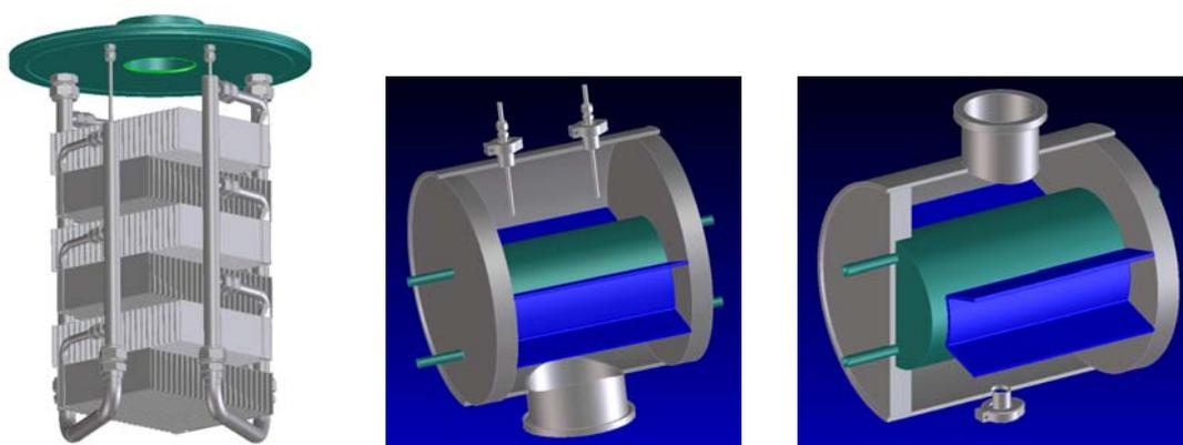
Figure 2.3 *Design drawings of the assembly of 6 plate-fin heat exchangers in the sorbent reactor (left), the plate-shell evaporator (middle) and the condenser (right). The green sections in the middle represent the plate area; the blue parts are support/separator plates*
