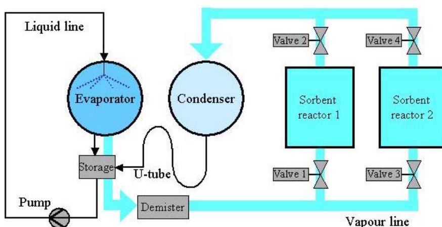
Figure 2.1 Basic system layout of the sorption cooling system
