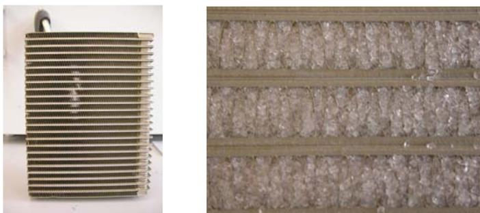
Figure 2.2 *Plate fin heat exchanger to be used as sorbent reactor (left) and detail of a silica-gel filled part of the heat exchanger (right)*
