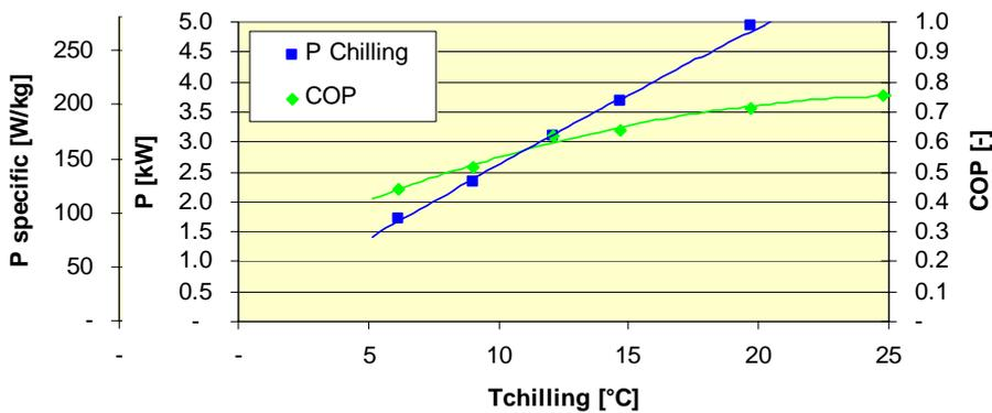
Figure 3.4 *(Specific) average chilling power and average COP as a function of the chilled water inlet temperature*
