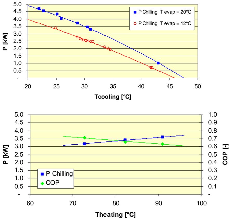
Figure 3.3 *Cooling power as a function of the cooling water inlet temperature at different chilled water ( $T_{evap}$ ) temperatures (first). Cooling power and average COP at different heat source inlet temperature (second)*
