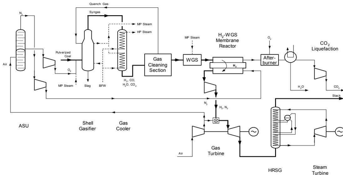
Figure 2 IGCC with H<sub>2</sub>-selective WGS-Membrane Reactor
