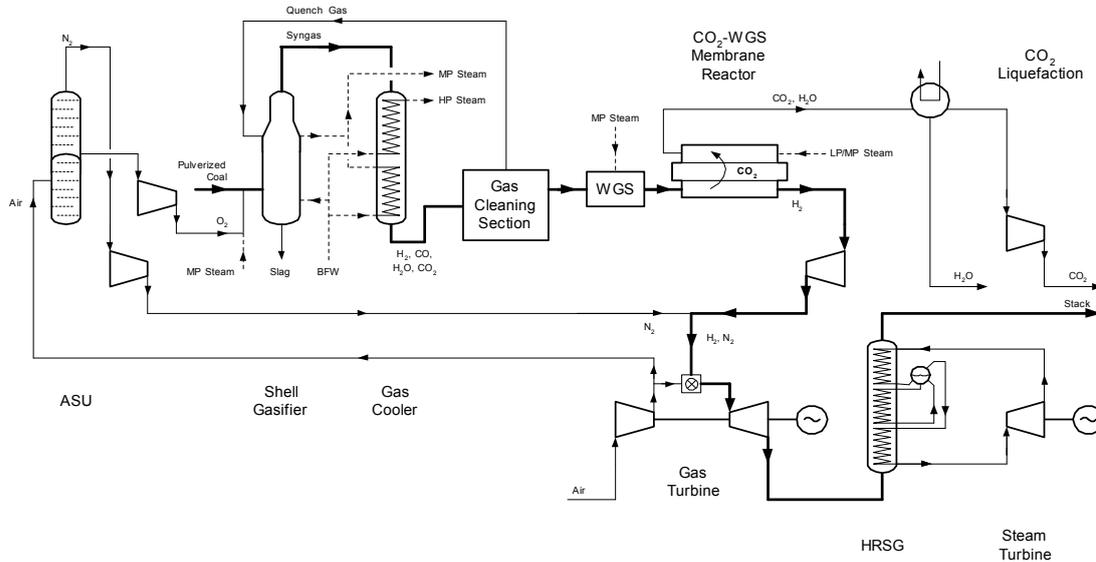
Figure 3 IGCC with CO<sub>2</sub>-selective WGS-Membrane Reactor
