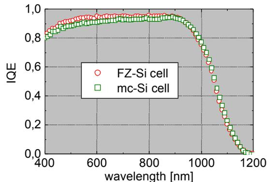
Figure 5. IQEs of FZ and mc-Si solar cell.
