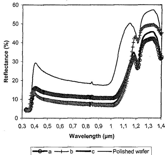
Fig 1: Lowest achieved encapsulated reflectances per etch type. a: Alkaline saw-damage etch on (110) orientation. b: Alkaline texture etch on (100) orientation. c: Acidic etch in pitted "tub" region (miscellaneous orientation).
