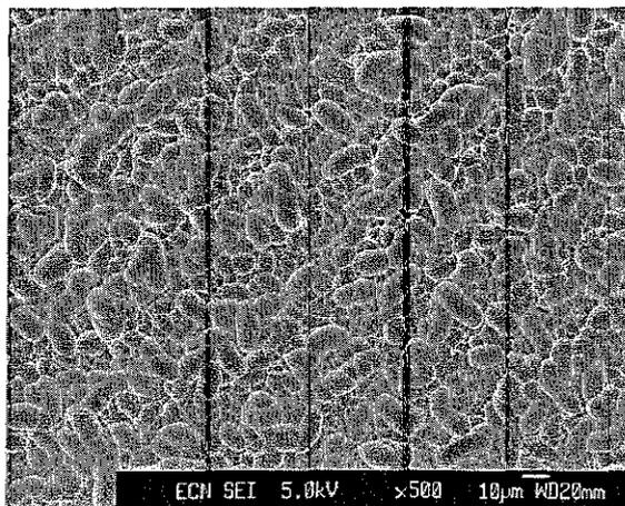
Fig. 2: SEM picture of isotropic pitted texture on multicrystalline silicon
