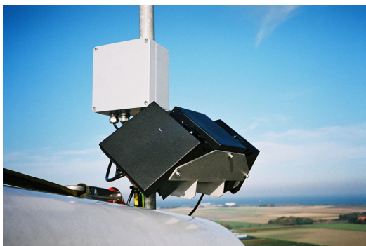
Figure 3: Infrared floodlights mounted on nacelle.
