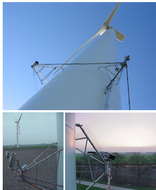
Figure 2: (upper) camera, rain sensor, infrared lights and WLAN antenna attached to tower, (left) camera at North side with four N80 turbines in line, (right) infrared lights at West side.
