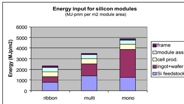
**Figure 8:** Comparison of typical energy input for manufacturing of various types of crystalline-silicon modules, situation 2005 [3].
