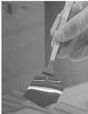
**Figure 5:** Lift-off silicon film (photo IMEC).
