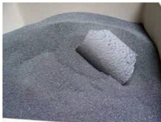
**Figure 3:** Granular solar grade silicon feedstock before melting and subsequent directional solidification to form a multicrystalline silicon ingot (photo Deutsche Solar).
