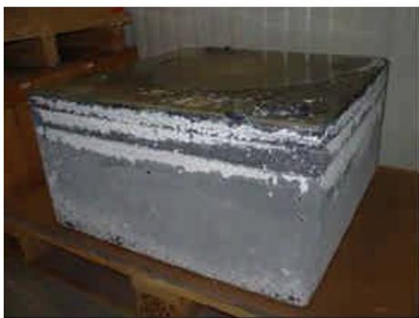
**Figure 4:** Newly made 400 kg multicrystalline silicon ingot (photo Deutsche Solar).
