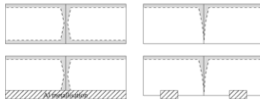
Figure 5: Shunt formation mechanism because of phosphorous diffusion. The left hand side applies to the standard process, the right hand side to the shunt free process. Top row is after phosphorous diffusion, bottom row after alloying the rear side metallisation.
