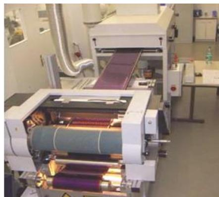
**Figure 1:** Roll-to-roll production line at VHF-Technologies.
