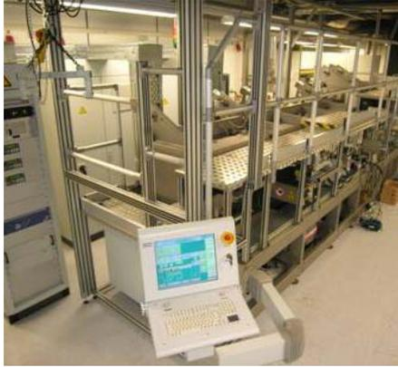
**Figure 2:** New MW-PECVD roll-to-roll system built by the system manufacturer R&R and shipped to ECN
