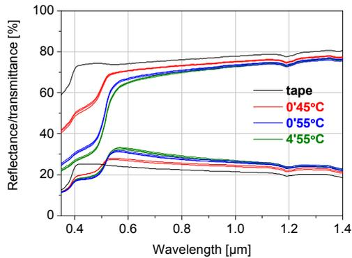
**Figure 4:** UV-VIS spectra of CdS layers on glass beads
