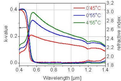
**Figure 5.** k-value and refractive index calculated from optical spectra
