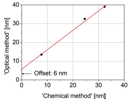
**Figure 6:** Relationship between the CdS layer thickness on glass beads determined by the optical and chemical method
