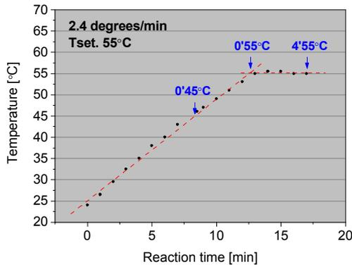
**Figure 1:** Cold start CdS deposition process and highlighted: three conditions chosen for this work
