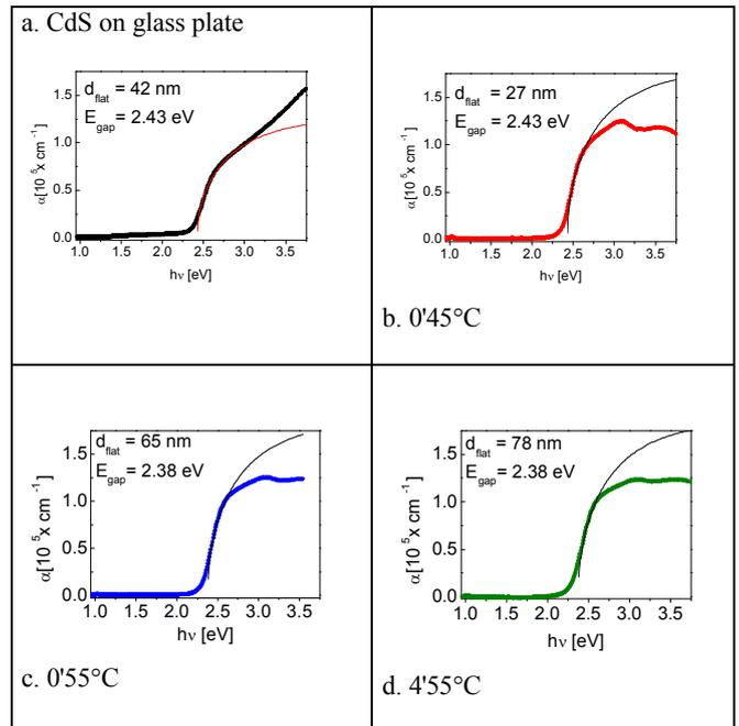
**Figure 3:** Bandgap determination for CdS layer on a microscopic glass plate (a) and CdS layers on glass beads: sample 0'45°C (b), 0'55°C (c) and 4'55°C (d) (flat) is the layer thickness determined using the thin layer configuration on flat substrates, for glass beads see section 3.2.1)
