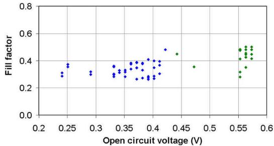
**Figure 7:** Fill factor and open circuit voltage determined for CuInS<sub>2</sub> bead cells (each measurement has performed on an area of 0.08 mm<sup>2</sup>, covering approximately 20 beads); Effective CdS layer thickness 34 nm (blue dots) and 39 nm (green dots)
