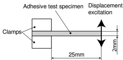
**Figure 2:** Set-up of the characterisation experiments.
