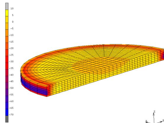
**Figure 18:** Normal stress distribution in a 200µm thick adhesive interconnect after cooling down from 150°C.
