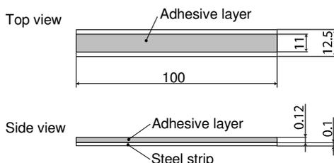
**Figure 7:** Dimensions of the adhesive on strip sample after curing of the adhesive layer. All dimensions are in mm.
