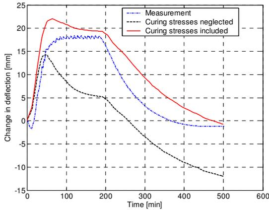
**Figure 10:** Comparison between measured and calculated lateral deflection change of the sample during temperature changes. Maximal oven temperature is nearly  $100^\circ\text{C}$ .
