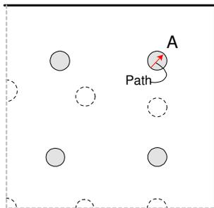
**Figure 15:** Path along the centre of the adhesive interconnect A (see Figure 14) for which stresses are plotted in subsequent figures. Perpendicular to the plane of drawing, the path is located in the mid-plane of the interconnect.
