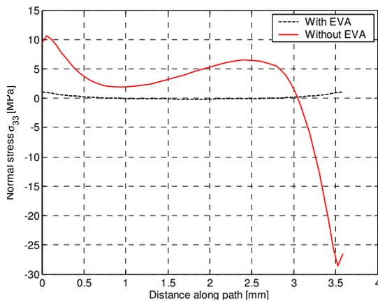
**Figure 20:** Normal stress in the adhesive interconnect after a temperature increase from 80°C to 150°C for a situation with and without EVA.
