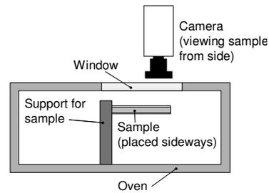
**Figure 8:** Set-up for measuring the deflection during temperature changes.
