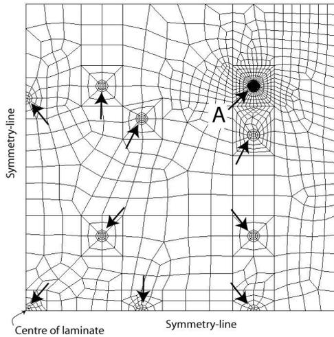
**Figure 14:** Top view of the 3D finite element mesh. The locations of the adhesive interconnects are indicated with arrows.
