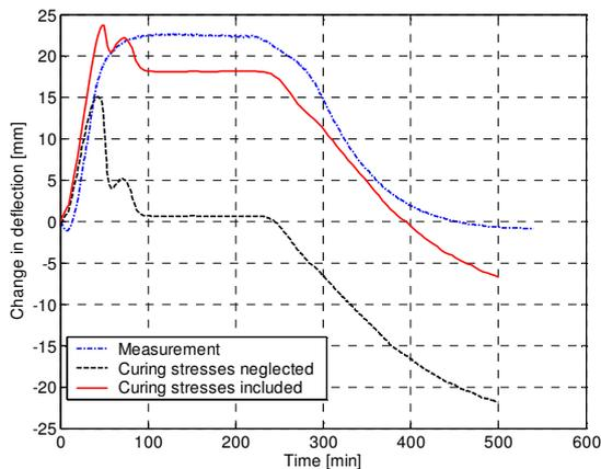
**Figure 11:** Comparison between measured and calculated lateral deflection change of the sample during temperature changes. Maximal oven temperature is nearly  $150^\circ\text{C}$ .
