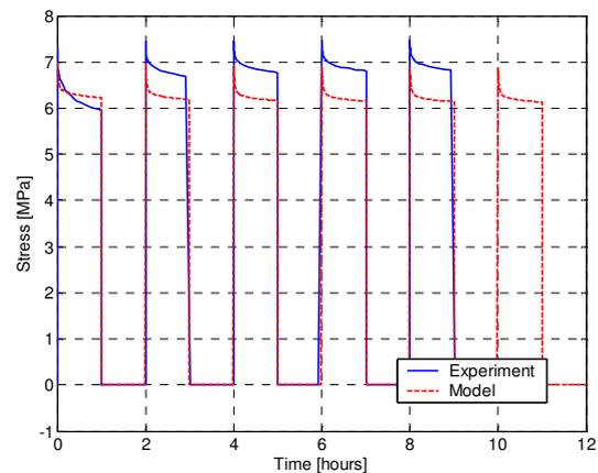
**Figure 5:** Comparison between model predictions and experiments for a repetitive relaxation experiment at -20°C.
