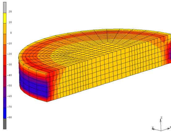
**Figure 19:** Normal stress distribution in a 500µm thick adhesive interconnect after cooling down from 150°C.
