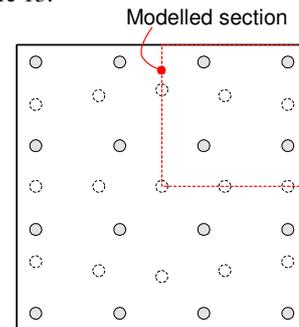
**Figure 12:** Top view of the single cell laminate as studied by means of numerical simulations. Circles denote the location of adhesive interconnects.
