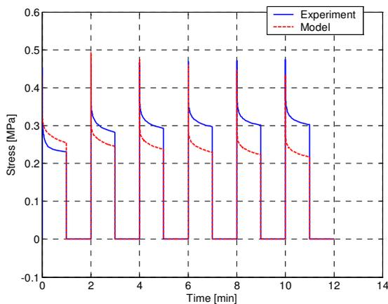
**Figure 6:** Comparison between model predictions and experiments for a repetitive relaxation experiment at 120°C.
