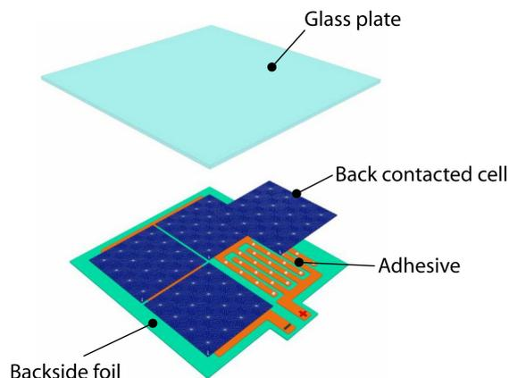
**Figure 1:** Layout of a PV module incorporating electrically conductive adhesive interconnects.
