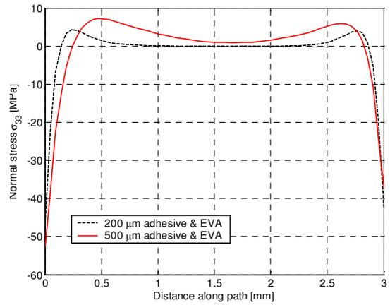
**Figure 16:** Normal stress in the adhesive along the path shown in Figure 15 after cooling down from 150°C to 20°C.
