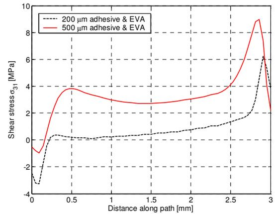
**Figure 17:** Shear stress in the adhesive along the path shown in Figure 15 after cooling down from 150°C to 20°C.
