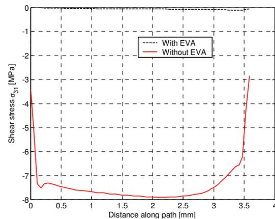
**Figure 21:** Shear stress in the adhesive interconnect after a temperature raise from 80°C to 150°C for a situation with and without EVA.
