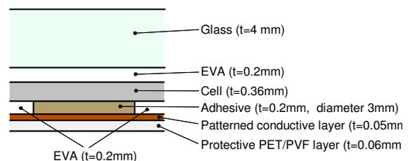
**Figure 13:** Cross-section of a part of the single cell laminate. The symbol  $t$  denotes the thickness of a layer.
