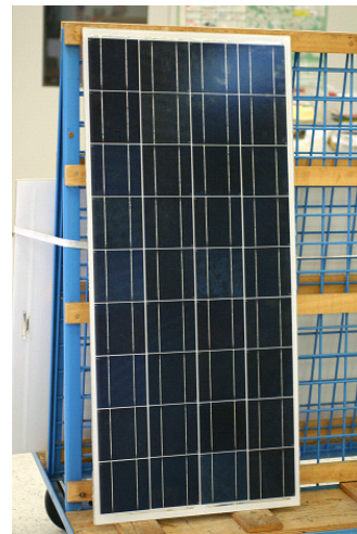
Figure 6: Full size module with screen-printed cells and an encapsulated cell efficiency of 16.8%.
