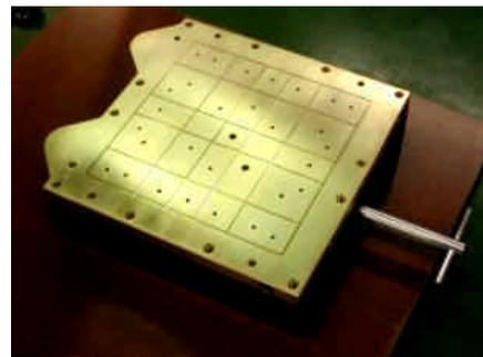
**Figure 3:** Photograph of the PUM measurement chuck. Current probes (16 to the emitter terminals and 15 to base terminals) contact the cell from the rear.
