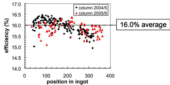
**Figure 2:** Efficiencies of ECN baselines made in a period of 2 years.
