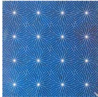
**Figure 1:** Photograph of a 225 cm<sup>2</sup> back-contacted PUM cell. The emitter contacts at the rear are realized through 16 laser-drilled vias. Interconnection can be realized at the rear, which makes pick-and-place module manufacturing possible. Furthermore the resistance losses in the module will be very small because of full interconnection from the rear. More details can be found in [1,2].
