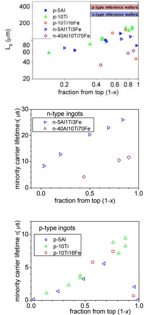
**Figure 3:** Minority carrier diffusion length (determined from the internal quantum efficiency) and corresponding minority carrier lifetime. For the conversion from diffusion length to lifetime, the additional suppression of carrier diffusion in the n-type ingots by a factor 2-3 was taken into account.
