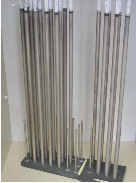
Figure 2.2 Set of membrane tubes with a length of 0.8 meter for the separator unit
