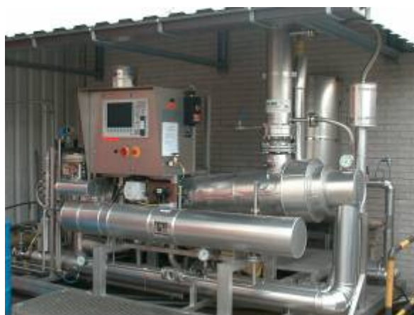
Figure 3.2 Pilot scale 1 m 2 membrane area pervaporation test system
