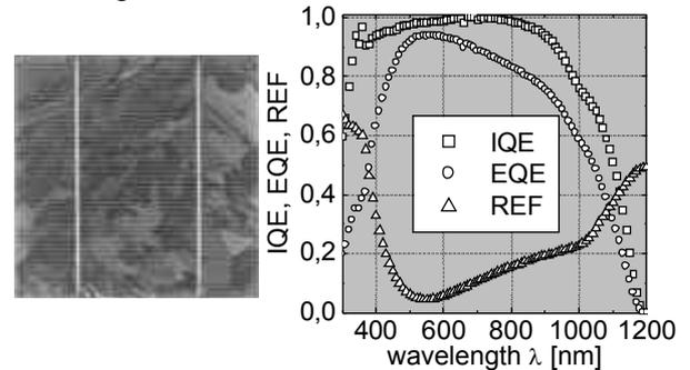
Figure 3 (left) 12.5x12.5 cm<sup>2</sup> n-type mc-Si solar cell and (right) spectral response measurement of this cell.
