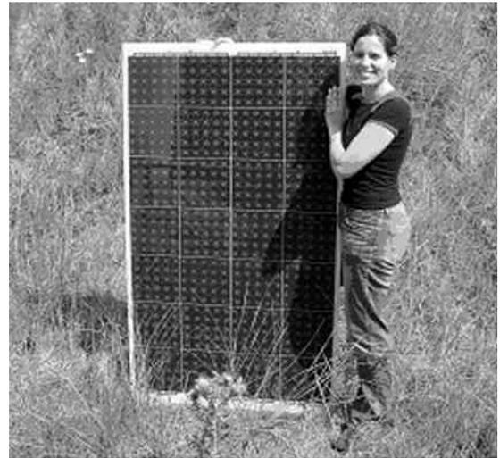
Figure 2. Completed 28 cells 8-inch module
