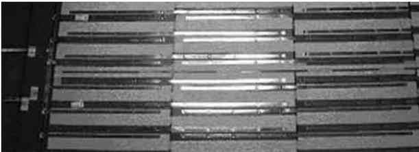
Figure. 1 Soldered back- contacted cells with insulation pads on rear side
