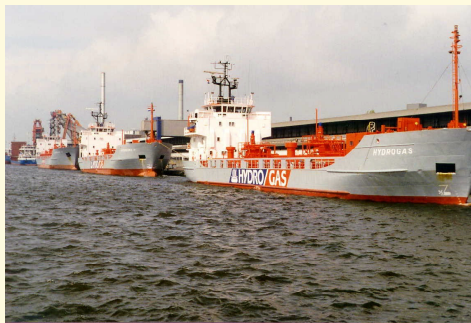
Hydro Agri CO 2 -tankers, approximately 1500 m 3 capacity
