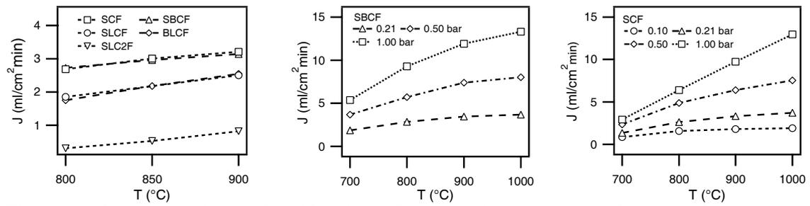
Figure 1: The oxygen fluxes of SLC2F, SCF, SBCF, SLCF, BLCF as a function of temperature (feed  $p_{O_2} = 0.21$  bar)(left); and those of SCF (middle) and SBCF (right) for different oxygen partial pressures at the feed side.
