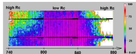
Fig. 4: Contact resistance mapping as function of wafer temperature. Temperature scale is not linear.
