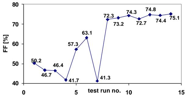
Fig. 6: Evolution of best FF results for test runs with different frits, pastes and using different settings.
