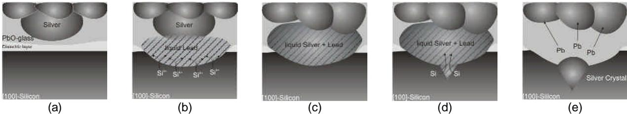
Fig. 1: Silver growth model. (a) Schematic cross section of Ag thick film paste on [100] silicon after burn-out. (b) Glass penetrated the dielectric layer → redox reaction between glass and silicon. (c) Silver particle dissolves in liquid lead. (d) Silicon interacts with liquid silver–lead alloy → formation of inverted pyramids. (e) Phase separation on cooling down → silver recrystallizes on <111> planes of the pyramid.
