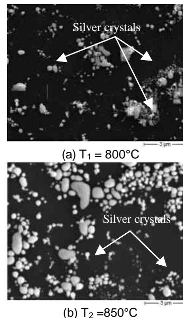
Fig. 2: SEM photographs of <100> FZ, chemically polished silicon surfaces with a 38 Ohm/sq. emitter. Samples were fired at different peak temperatures in an RTP-furnace. After firing silver fingers were etched off. Silver crystals are clearly visible (white). Number and size of crystals increase with increasing temperature.
