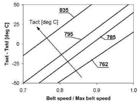
Fig. 3: Actual wafer temperatures as a function of furnace settings.
