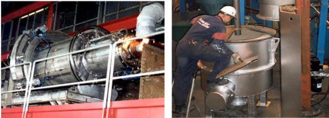
Figure 3. Solsilc pilot silicon metal production. SiC is formed in the plasma rotary furnace based on quartz and Carbon Black. Liquid silicon is produced from SiC and SiO<sub>2</sub> in an electric arc furnace.
