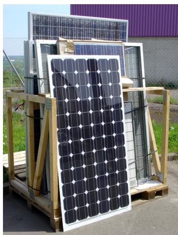
**Figure 1:** Disposed PV modules collected at Solar Materials, Deutsche Solar AG in Freiberg (Saxony, Germany). Valuable materials like the silicon solar cells, aluminium frame and encapsulation glass are recovered.
