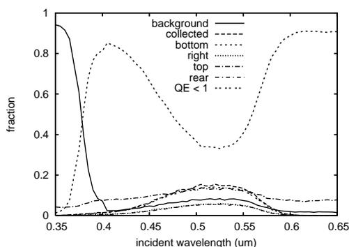
Figure 9: energy balance for the case without mirrors.
