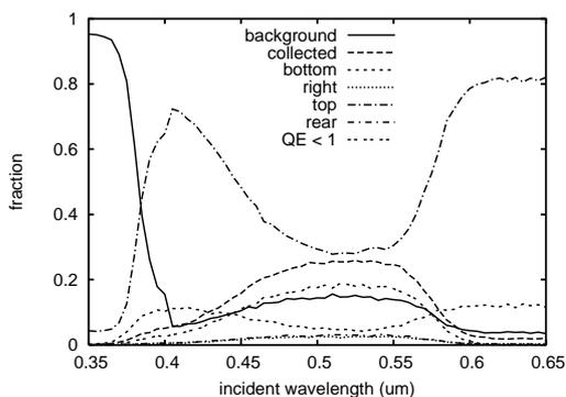
Figure 10: energy balance for the case with mirrors at Fr+Re+Ri and diffuse 85% mirror at bottom.
