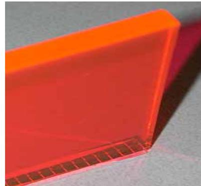
Figure 2: a multi-crystalline silicon solar cell fitted to a polymer slab.
