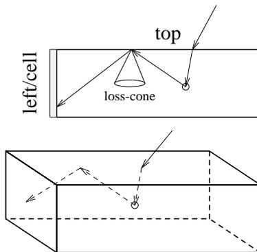
Figure 1: the luminescent concentrator: incident light is absorbed and re-emitted diffusely by luminescent particles in the polymer plate. The emitted light is transported to a solar cell at the left, the polymer plate acting as a wave guide.
