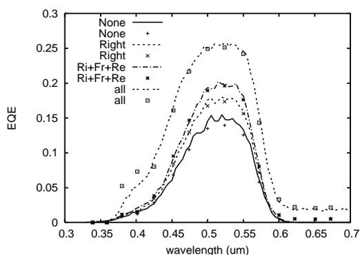
Figure 8 measured and calculated external quantum efficiency for different mirror configurations. *None* in the key means no mirrors, *all* means mirrors at all sides. Lines show the calculated EQE curves, markers show the measured ones.
