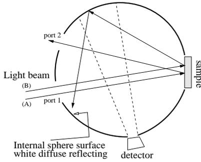
Figure 4: Integrating sphere layout for reflection measurements.
