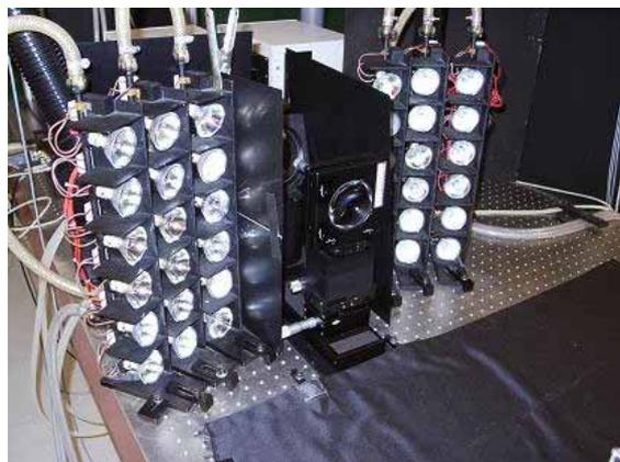
**Figure 2:** Illuminating the solar cell in the spectral responsivity setup at PTB: 36 halogen lamps are used for a uniform bias illumination, inbetween is the lens that projects the chopped monochromatic light onto the cell.
