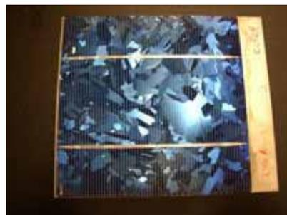
**Figure 1:** One of the reference cells used in the comparisons; it is glued on the metal mounting plate, this cell is 156 cm<sup>2</sup> in size.
