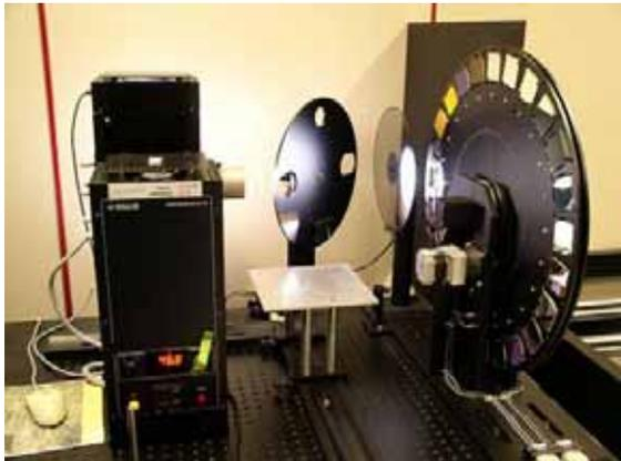
**Figure 4:** Filter monochromator setup at ECN. Above the measurement table (positioned outside the picture) a mirror is mounted to enable horizontal cell mounting.
