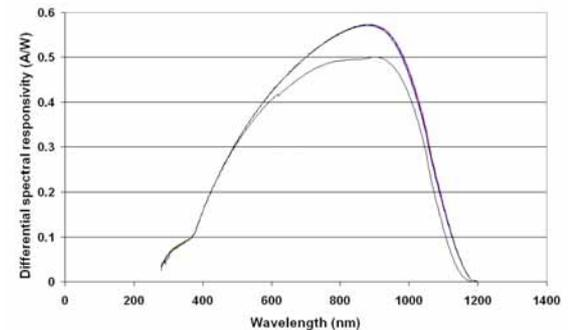
**Figure 6:** Absolute differential spectral responsivities for the 225 cm<sup>2</sup> cell at different bias levels. The levels are (in suns) 0.00001, 0.004, 0.041, 0.10, 0.26, 0.70 and 0.80, the spectral responsivity curves increase with bias level.
