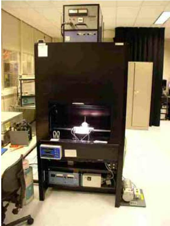
**Figure 3:** Solar simulator at ECN, used to measure the J-V curves for solar cells up to 225 cm<sup>2</sup> in size.
