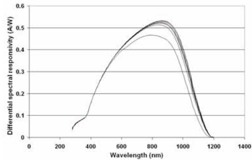
**Figure 5:** Absolute differential spectral responsivities for the 156 cm<sup>2</sup> cell at different bias levels. The levels are (in suns) 0.00001, 0.005, 0.052, 0.11, 0.38, 1.02 and 1.14, the spectral responsivity curves increase with bias level.
