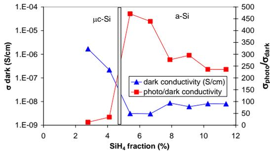
**Figure 9:** Dark and photoconductivity of a series of silicon layers grown with various  $\text{SiH}_4$  fractions.
