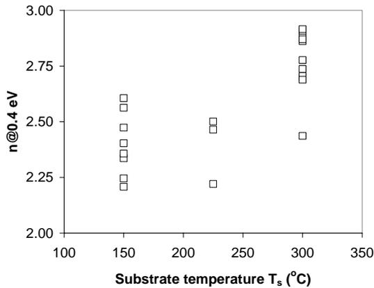
**Figure 2:** Refractive index of  $\mu\text{c-Si}$  as a function of substrate temperature  $T_s$ . Silane fraction was 5%. Scattering of the data is due to variation of the other deposition conditions.
