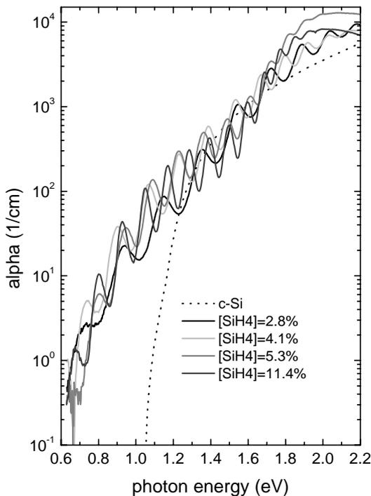
**Figure 10:** FTPS spectra of layers grown with various  $\text{SiH}_4$  fractions
