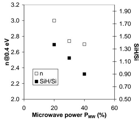
**Figure 4:** Refractive index determined by FTIR and emission intensities of  $\text{SiH}$  (414 nm) and  $\text{Si}$  (288 nm).
