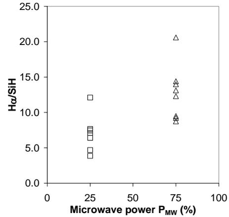
**Figure 3:** Ratio of  $\text{H}\alpha$  (emission at 656 nm) and  $\text{SiH}$  (emission at 414 nm) versus applied MW power. Silane fraction was 5%, other deposition conditions were varied.
