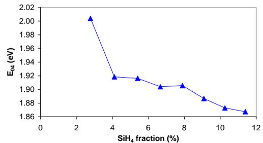
**Figure 8:** Bandgap E<sub>04</sub> of layers grown with various SiH<sub>4</sub> flows.
