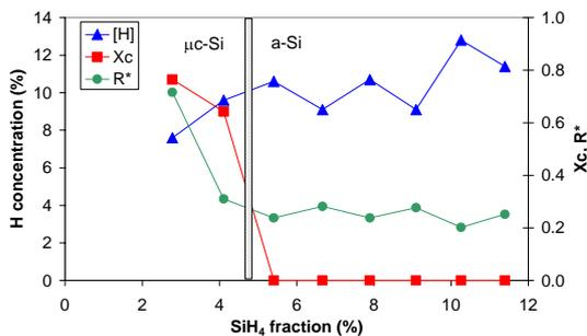
**Figure 6:** Hydrogen concentration and structure factor R\* for silicon layers grown with various SiH<sub>4</sub> flows. Crystalline fractions X<sub>c</sub> as determined by Raman spectroscopy have also been included.
