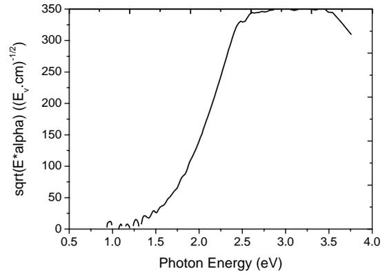
**Figure 7:** Typical example of  $\sqrt{\alpha E}$  of a microcrystalline/amorphous Si layer, obtained with R/T measurements.
