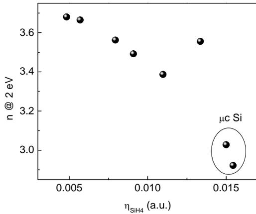
**Figure 5:** Refractive index of silicon layers versus the silane utilization efficiency  $\eta_{\text{SiH}_4}$  defined as growth rate/SiH<sub>4</sub> flow. The two samples on the right are microcrystalline silicon; the others are largely amorphous.
