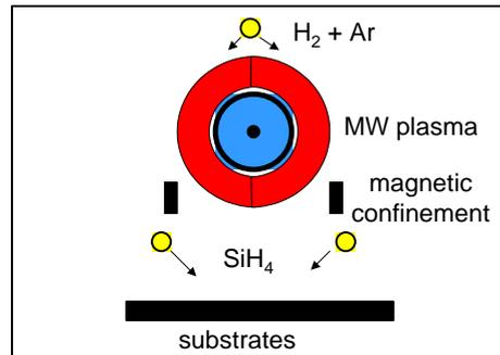
**Figure 1:** Cross section of linear microwave plasma source.
