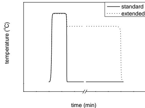
**Figure 1:** Schematic of the two different temperature profiles used for the phosphorus diffusion/gettering in this experiment; i) the standard gettering at a constant temperature, and ii) the extended gettering consisting of same temperature and duration as i) followed by an extended time at lower temperature. The investigated durations of the low-temperature tail were 45 minutes, 150 minutes, and 480 minutes.
