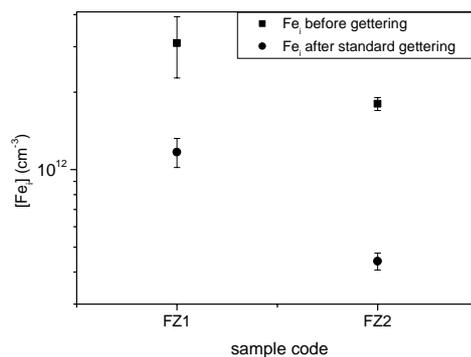
**Figure 4:** Interstitial iron concentration in two floatzone wafers with artificially in-diffused iron, after standard gettering and extended gettering.
