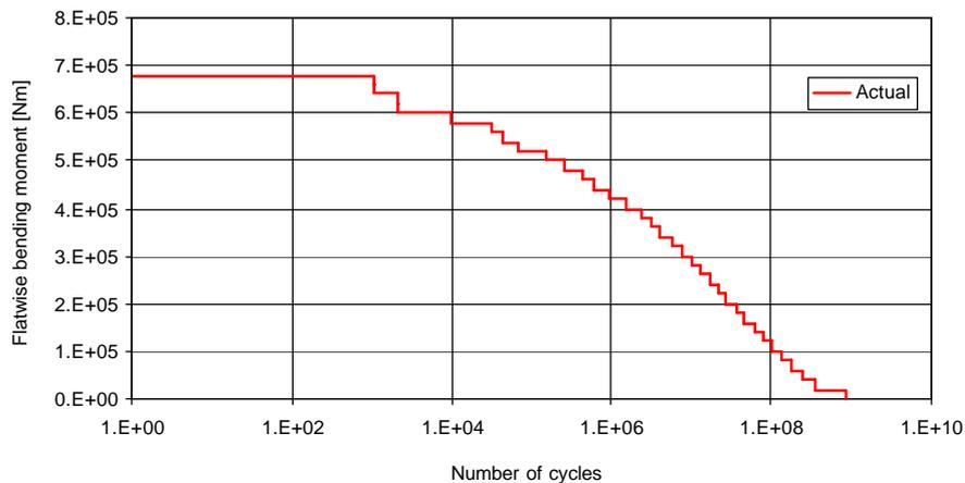
Figure 8: Example of load spectrum of flap wise bending moment
