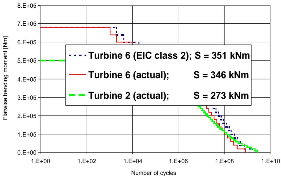
Figure 11: Three load spectra reduced to three equivalent loads
