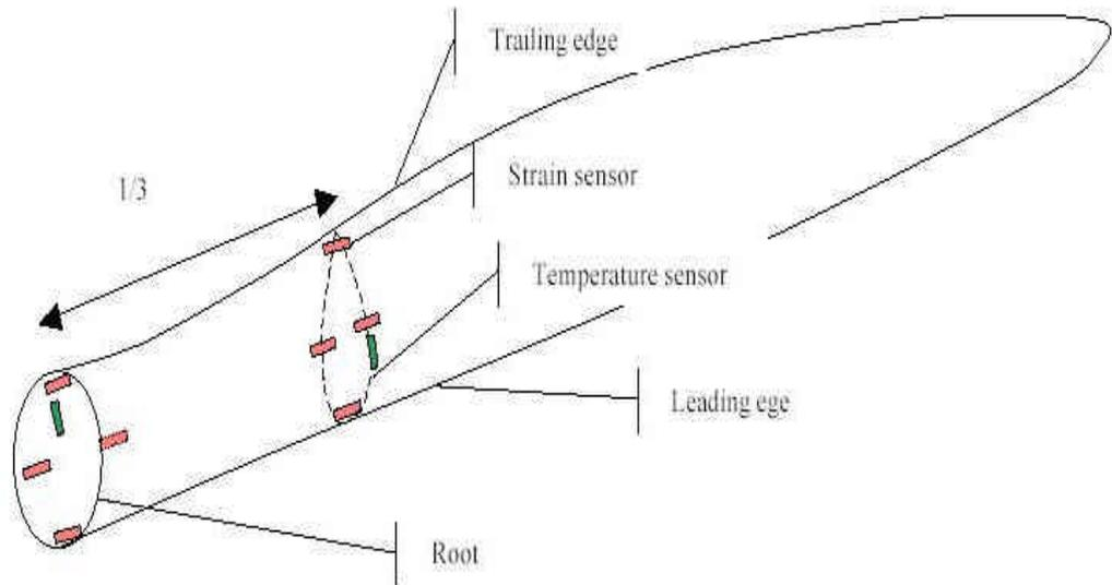
Figure 1: Strain sensor configuration in wind turbine blade
