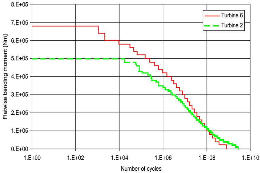
Figure 10: Example of comparison between the fatigue loads of two wind turbines within one wind farm
