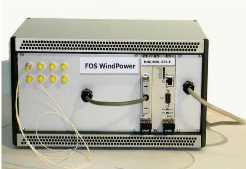
Figure 3: Fiber optic rotor module for eight lines
