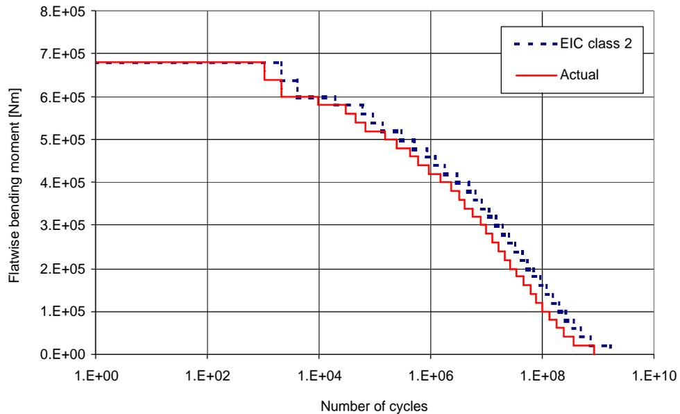
Figure 9: Example of comparison between actual load spectrum and load spectrum in accordance with the design wind conditions (in this case IEC class 2)
