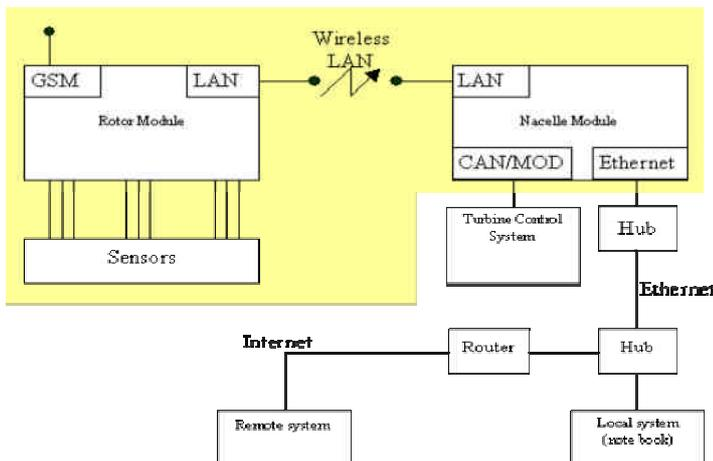
Figure 4: Blade condition monitoring configuration
