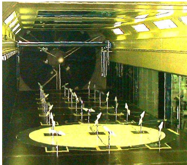
Figure 4: In the boundary layer tunnel of TNO, first measurements with a 1:400 scaled model of a wind farm confirmed Heat and Flux.
