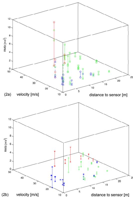
Fig. 2: Impact energy vs. distance to sensor and speed. colors: blue-green-red: increasing mass symbols (2a):  $\square$  frontal,  $\circ$  frontal-suction side, symbols (2b): \* grazing, + suction side, x pressure side
