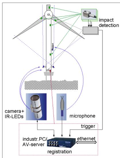
A new monitoring system for registration of bird collisions, WT-BIRD, has been developed at ECN [5]. It uses video cameras and microphones combined with event triggering by sound and vibration measurements. Figure 1 shows a schematic overview of the system.
