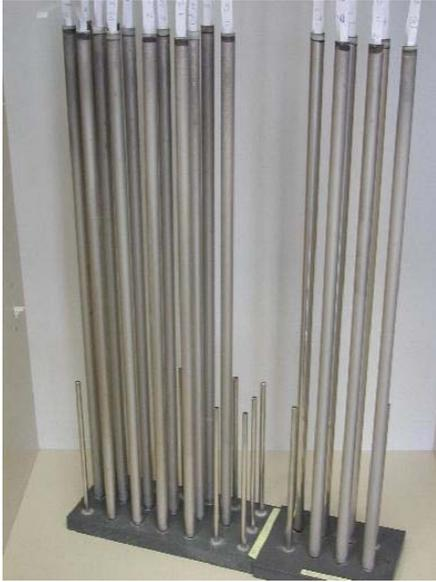
Figure 1.2 Set of 24 membrane tubes with a length of 0.8 meter for the separator unit
