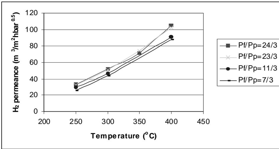
Figure 4.1 Hydrogen permeance at different temperatures ( $P_f$ = feed pressure,  $P_p$ =permeate pressure, pressures in barg)
