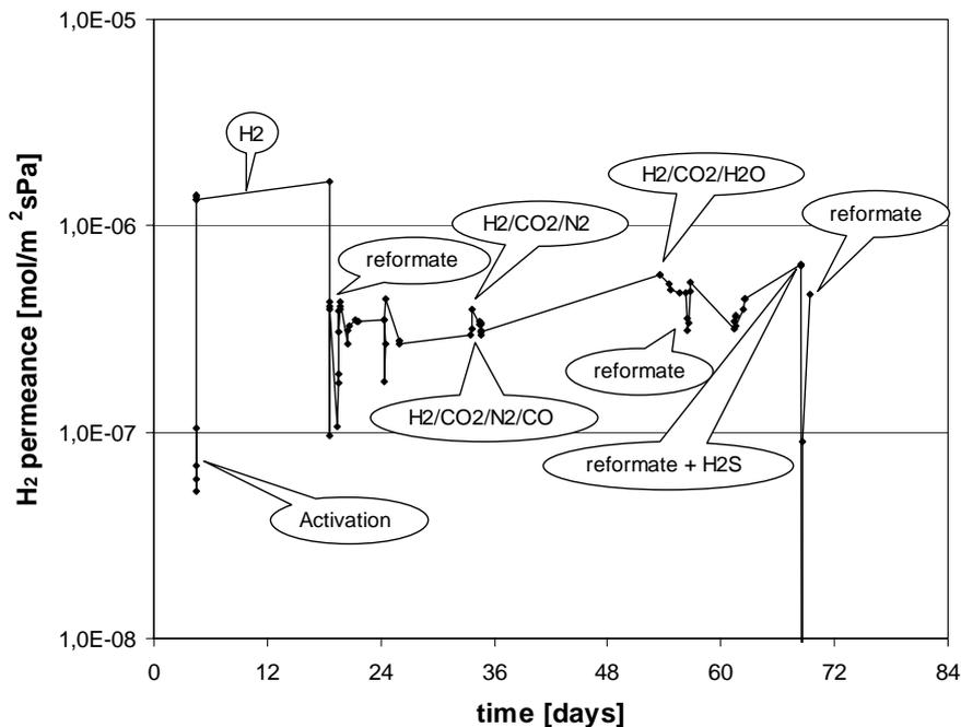
Figure 4.2  $H_2$  permeance vs. time on stream ( $T=350^\circ\text{C}$ ,  $P_{\text{feed}}= 23 - 45 \text{ bara}$ )
