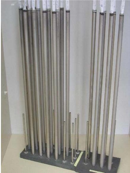
Figure 3.2 *Set of membrane tubes with a length of 0.8 meter for the separator unit*
