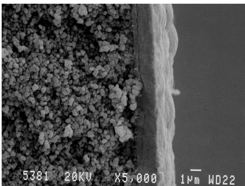
Figure 3.1 SEM cross section of fractured sample of Pd/23%Ag membrane layer on ceramic support
