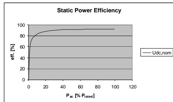
Figure 1, Static power efficiency versus ac power, measured on the second prototype
