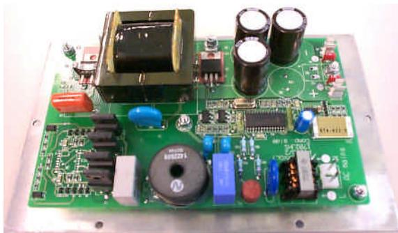
Picture 1, the second prototype of the PV2GO inverter without enclosure
