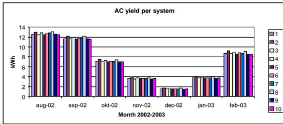
Figure 2, AC Yield per system, measured at Petten in The Netherlands
