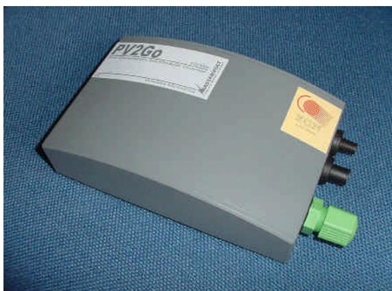
Picture 2, the second prototype of the PV2GO inverter
