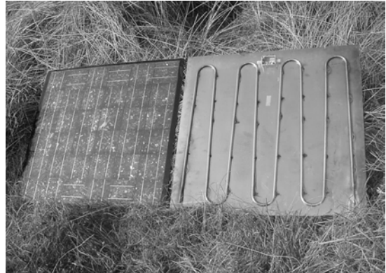
Figure 1: Front and back of a PVT laminate
