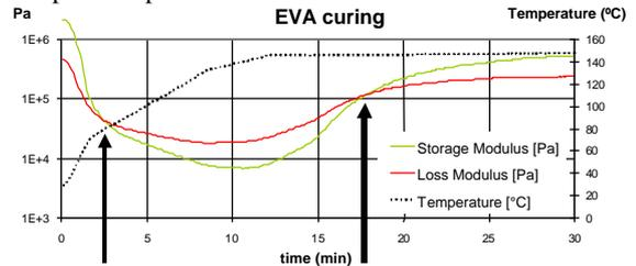
**Figure 8:** DMA test of EVA under lamination-cycle temperature conditions. The arrows indicate solid-to-fluid and fluid-to-solid transitions.
