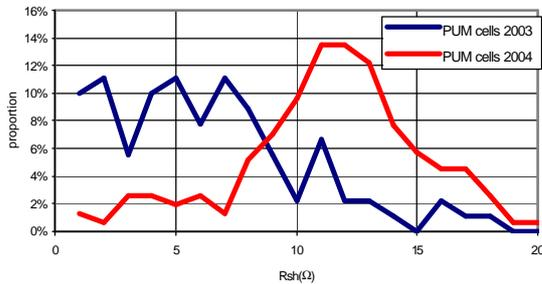
**Figure 2:** Shunt resistance distribution of  $225\text{ cm}^2$  PUM cells with  $330\mu\text{m}$  thickness (bin size  $1\Omega$ ).
