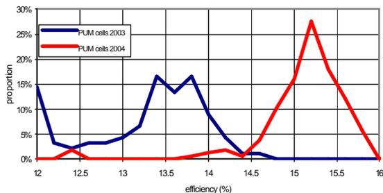
**Figure 3:** Efficiency distribution of  $225\text{ cm}^2$  PUM cells in 2003 and 2004 (bin size 0.2%).
