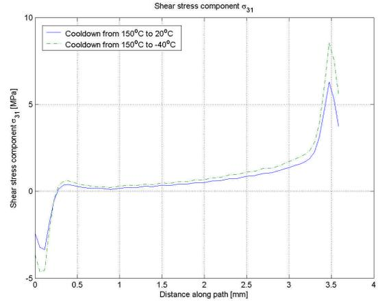
**Figure 7:** Shear stress FEM analysis on an adhesive interconnection spot in a 4x9 module.
