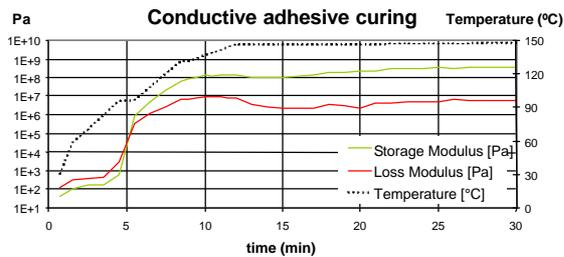
**Figure 9:** DMA analysis results on commercial available adhesive.
