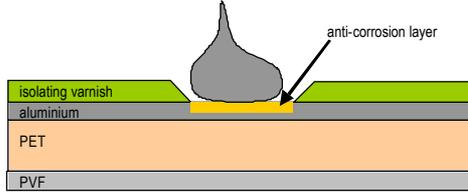
**Figure 6:** Overview of the layers in a back-sheet foil, and how it is modified into an interconnection foil.
