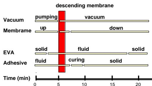
**Figure 10:** Lamination processing sequence versus time.
