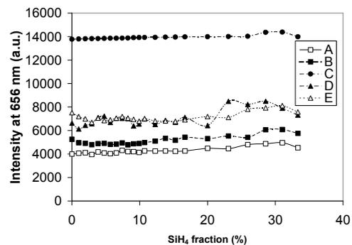
**Figure 9:** Light intensity emitted by H<sub>α</sub> at 656 nm for different configurations.
