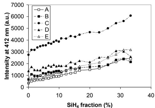
**Figure 8:** Light intensity emitted by SiH\* at 412 nm for different configurations.
