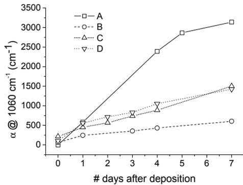
**Figure 5:** IR absorption of Si-O bonds at 1060 cm<sup>-1</sup> as a function of time.
