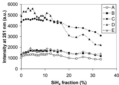
**Figure 6:** Light intensity emitted by Si\* at 251 nm for different configurations.
