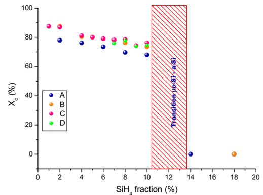
**Figure 4:** Crystal fractions of layers deposited in various MW source geometries.
