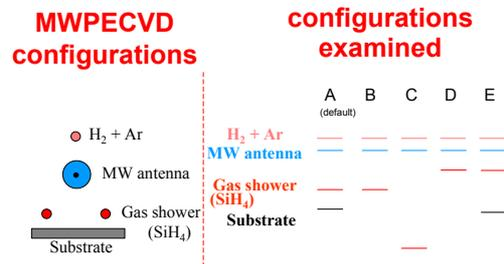
Figure 1: Micro-wave plasma source configurations.
