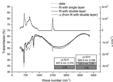
**Figure 3:** Fit of typical FTIR spectrum of  $\mu\text{c-Si}$  layer with single and double layer model.
