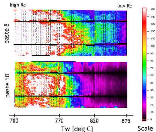
**Figure 6:** Contact resistance mappings as function of wafer temperature for pastes 8 and 10. Temperature scale is not linear.
