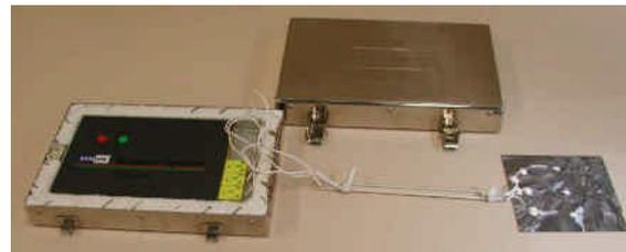
**Figure 1:** Data logger placed in opened thermal barrier with TCs attached to a wafer as used in [2].
