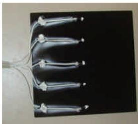
Figure 2: Wafer with 5 K-type thermocouples.
