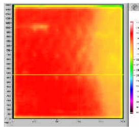
Figure 3: Voc map at setting CBM (full scale 450 - 620mV)
