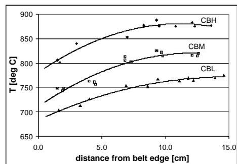
Figure 4: Cross belt temperature distribution at one belt speed for three peak zone temperatures.
