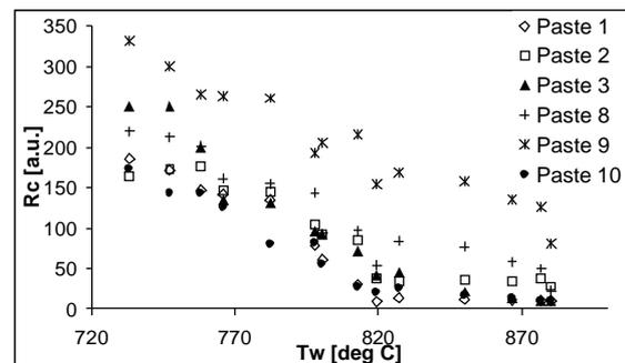
**Figure 7:** Local contact resistance as function of measured wafer temperature for pastes 1, 2, 3, 8, 9, and 10.
