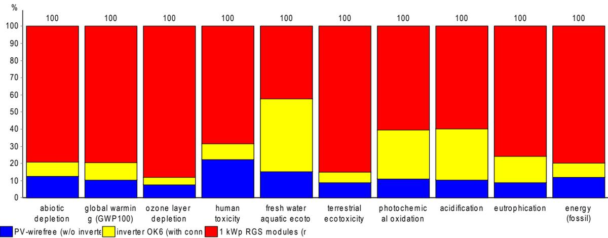
Analyzing 1 p assembly '1 kWp sys Wirefree/RGS'; Method: CML 2 baseline 2000 all +energy (w/o mar.ecotox) / World, 1990 / characterisation
