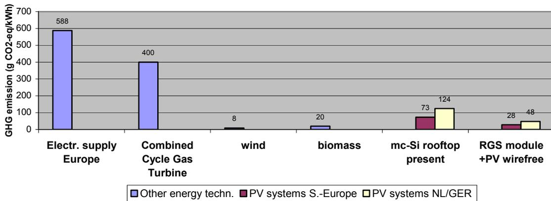
**Figure 4:** Greenhouse gas emissions for a kWh of electricity from different sources. The grid-connected PV systems are located either in Southern-Europe (1275 kWh/kWp/yr output) or in the Netherlands/Germany (750 kWh/kWp/yr).
