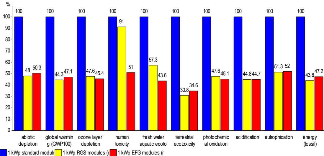
Comparing 1 p assembly '1 kWp standard modules (nf)' with 1 p assembly '1 kWp RGS modules (nf)' and with 1 p assembly '1 kWp EFG modules (nf)'; Method: CML 2
