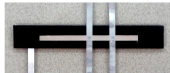
**Figure 8:** CISCuT cell with two front side aluminium tabs on 3 $\mu\text{m}$  aluminium to control the electrical contact at ultrasonic weld
