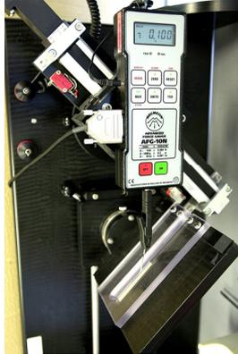
The shear or peel strength are determined using a test facility with adjustable angle between 0 and 45° (see Fig. 2) with a maximum strength of 10 N.
