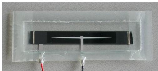
**Figure 3:** Connected and encapsulated CISCuT cell: with sputtered NiAl busbar
