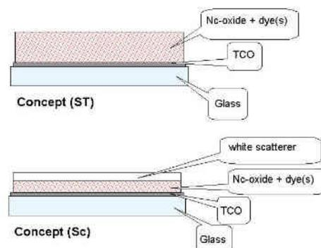
**Figure 1.** Schematic presentation of two nc-DSC concepts under investigation. The counterelectrodes are not shown for clarity.
