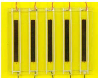
**Figure 2.** "Masterplate" containing five single nc-DSC with an active area of  $50 \times 5 \text{ mm}^2$ .
