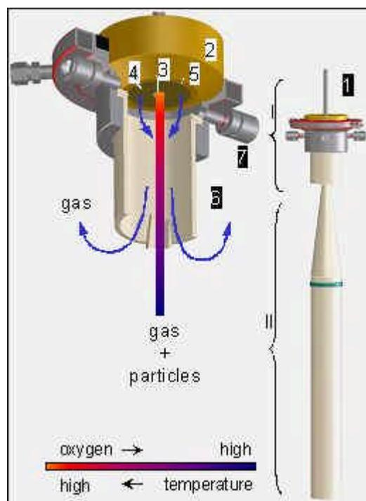
Figure 3. Schematic of the new Lab-scale Combustion Simulator. Legend: I Devolatilisation zone; II Combustion zone; 1 Solid fuel feed; 2 Flat flame gas burner; 3 Inner burner; 4 Outer burner; 5 Shield gas ring; 6 Reactor tube; 7 Optical access.
