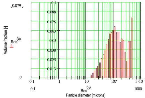
Figure 1. Left: sieve fraction  $>180 \mu\text{m}$  taken from a blend of Polish pulverised coal with 10% wood particles; right: the large wood particles result in a bimodal size distribution of the whole blend.
