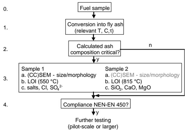
ash deposition tests developed earlier, are currently being integrated into an overall empirical biomass co-firing assessment method, the so-called Co-firing Assessment Tool (CAT).
