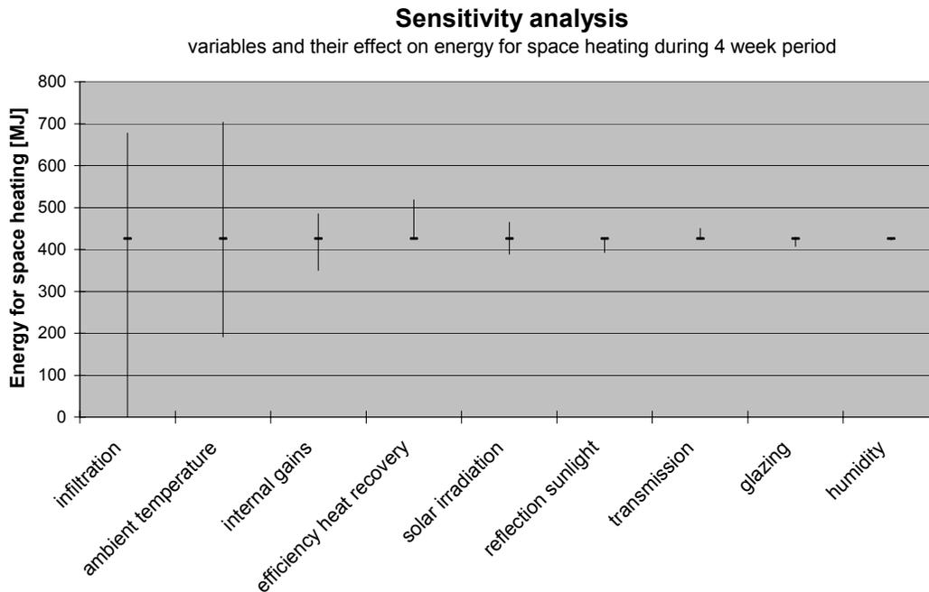
**Figure 4: Effects of realistic variations in variables on space heating demand for the validated model of Ecobuild test house B**
