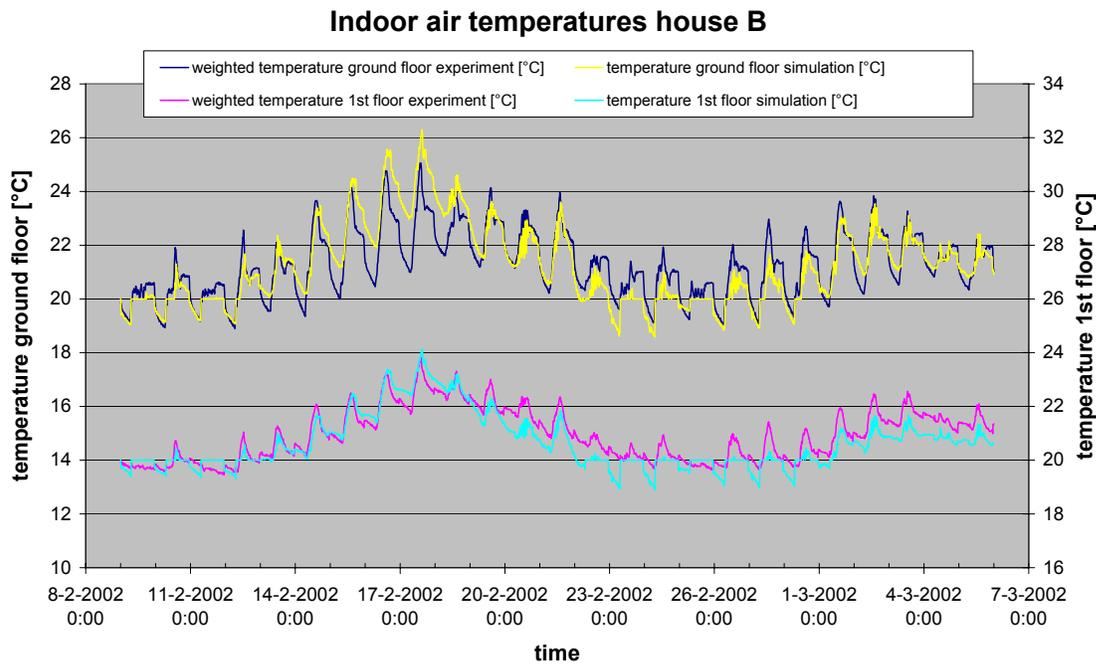
**Figure 3: Comparison of measured and simulated indoor air temperatures in house B**
