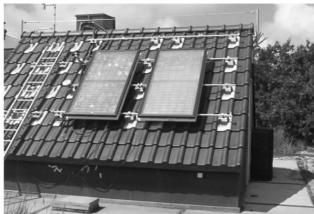
Figure 2 – Two PVT collectors, installed on the PVT test facility at ECN.
