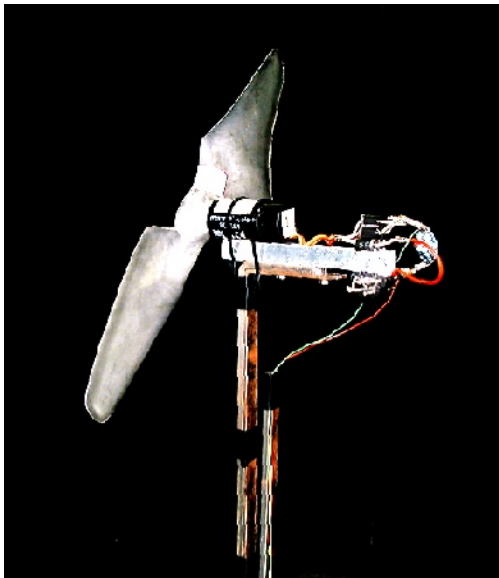
Figure 4 Wind turbine model, 25 cm diameter, NACA 0009 airfoils, 4 pitch settings.
