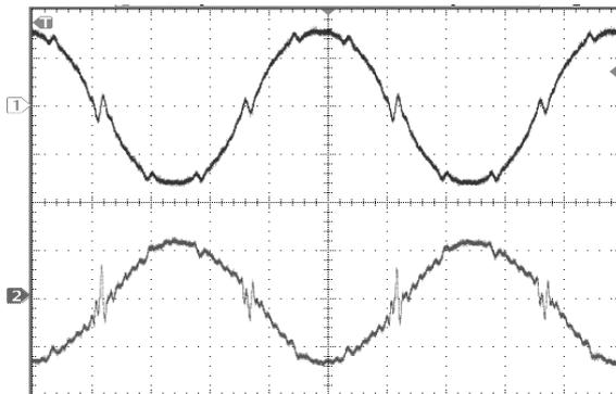
Fig. 8: Measurement on a maximum polluted grid without impedance. 1: grid simulator voltage (U3), 2: inverter current (I1).
