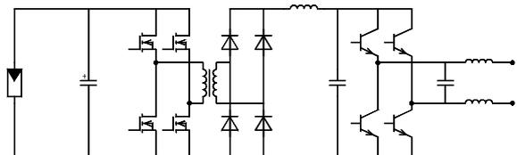
Fig. 2: Multi-stage high-frequency transformer H-Bridge PWM Converter with low-frequency unfolding bridge
