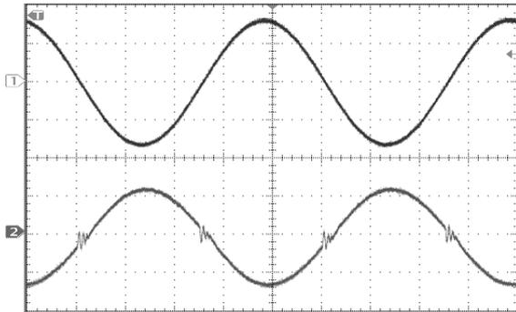
Fig. 6: Measurement on a clean grid without impedance.
