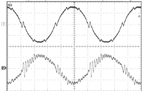
Fig. 11: Measurement on a maximum polluted grid with impedance.
