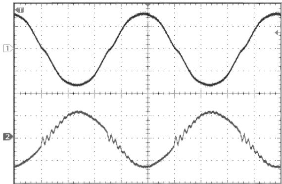
Fig. 10: Measurement on an average polluted grid with impedance.
