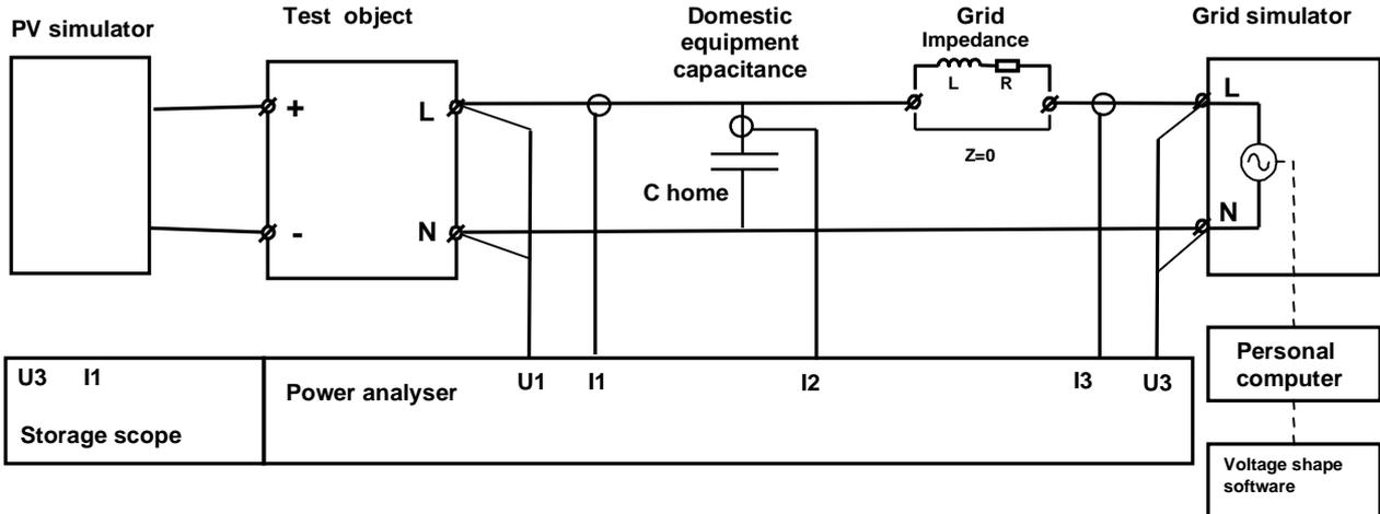
Fig. 3, Test set-up for the laboratory measurements.
