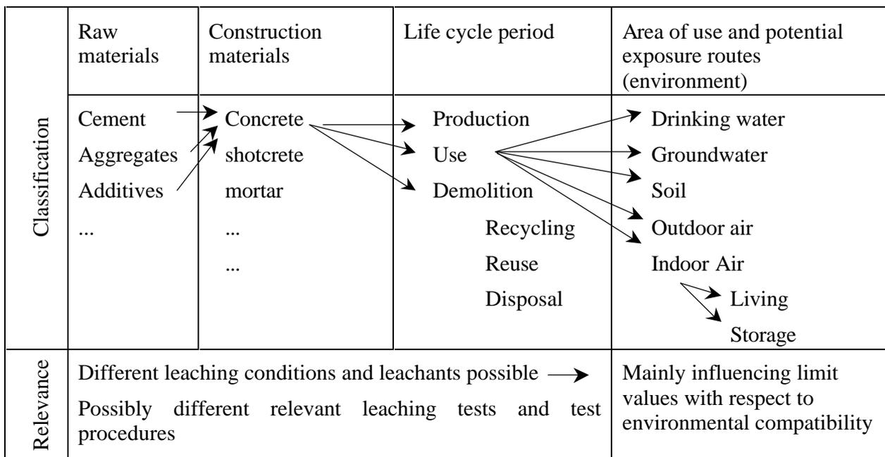
Figure 2. Environmental compatibility of cement-based materials (basic scheme)(Schiessl and Hohberg 1995, Van der Sloot et al, 1997).
