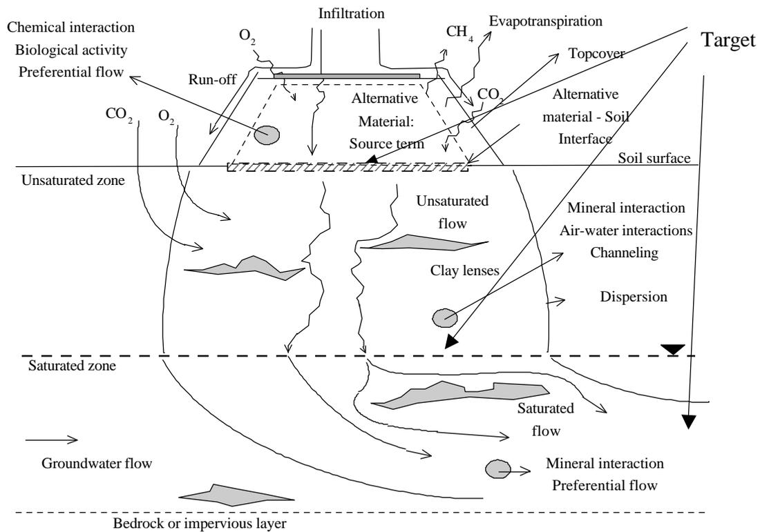
Figure 1. Schematic representation of release from “alternative” construction materials with the possible targets (surficial soil, subsoils, groundwater) for evaluation of environmental impact.
