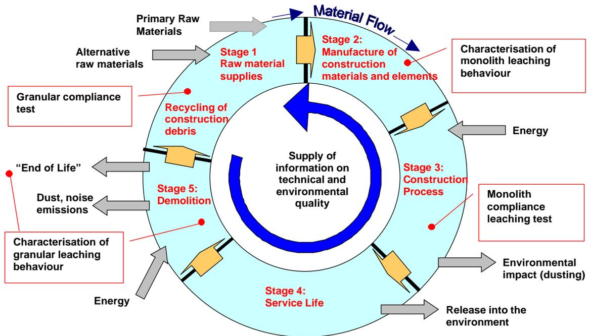
Figure 3. Life cycle stages of alternative materials in construction with characterisation and compliance leaching tests allocated to the different stages. (Modified after Rilem 22, 2000).
