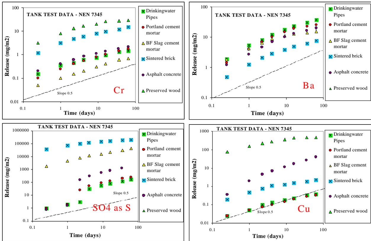
Figure 6. Cumulative release curves as a function of time for a wide range of monolithic materials as obtained by NEN 7345(1995).
