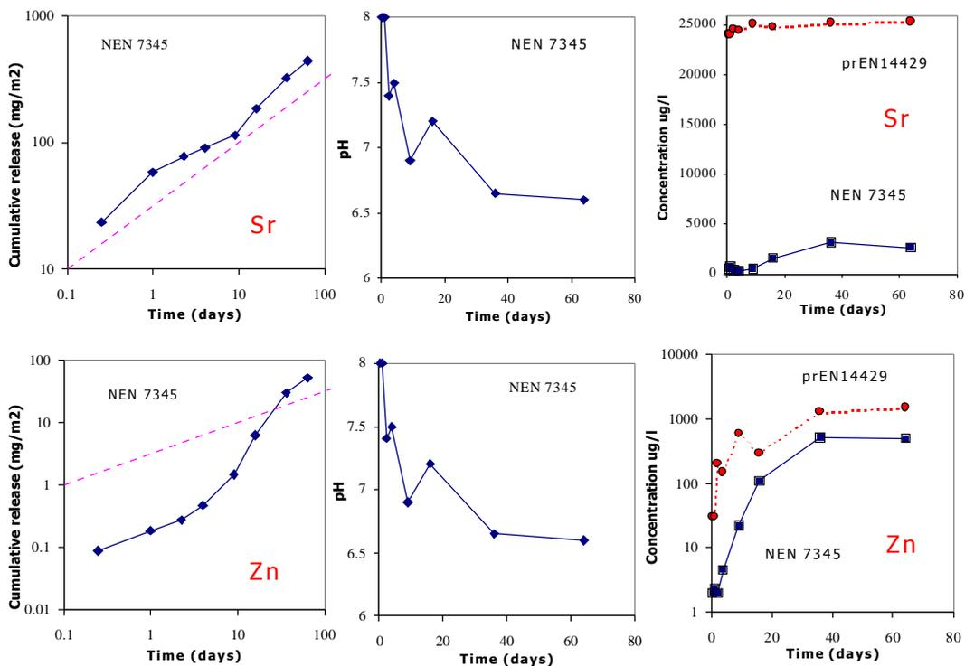
Figure 5. Cumulative release of Sr and Zn from cement-based material, pH variation during the test and concentration in eluate in relation to pH dependence test data at corresponding pH.
