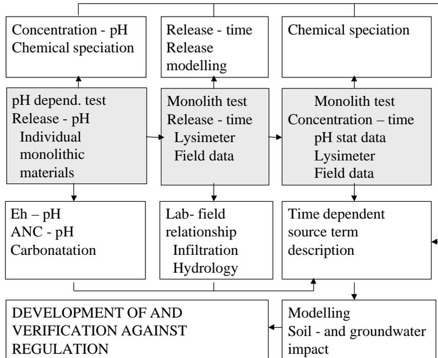
Figure 4. Scheme showing interrelations between test for monolithic materials, data processing and evaluation aspects for monolithic construction materials.
