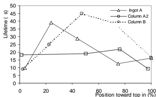
Fig. 1 Minority carrier lifetime in as cut wafers along columns of A and B ingots.
