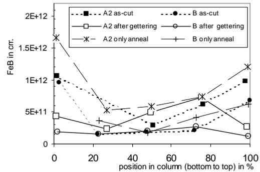
**Fig. 5** Distribution of FeB in wafers along the ingots A<sub>2</sub> and B before and after phosphorus gettering at 890°C for 12 min.
