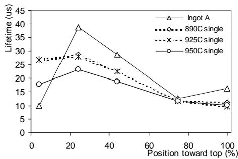
**Fig. 8** Lifetime after emitter diffusion (12 minutes at varying temperatures), as a function of position in the column for ingot A.
