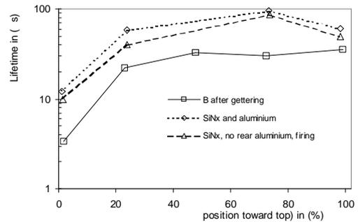
**Fig. 9** Minority carrier lifetime along the ingot B: effect of phosphorus gettering and Al rear side on the hydrogen passivation. Diamonds: co-firing of SiNx with Al rear side metallisation. Triangles: firing of SiNx without Al rear side.
