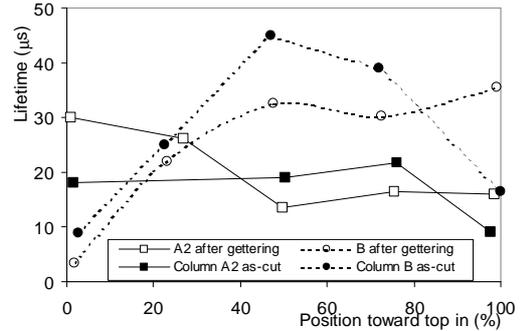
**Fig.4** Minority carrier lifetime before and after phosphorus gettering at 890°C for 12 min in wafers along the ingots A<sub>2</sub> and B.
