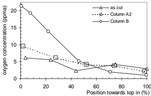
**Fig. 3** Distribution of oxygen in as cut wafers along the column of ingots A and B.
