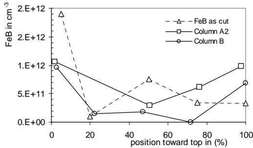
**Fig.2** Distribution of FeB in as cut wafers along columns of ingots A and B.
