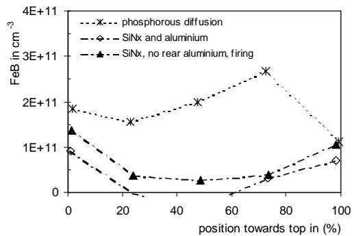
**Fig. 10** Change of FeB concentration along the ingot B after passivation. Same wafers as in Fig. 9.
