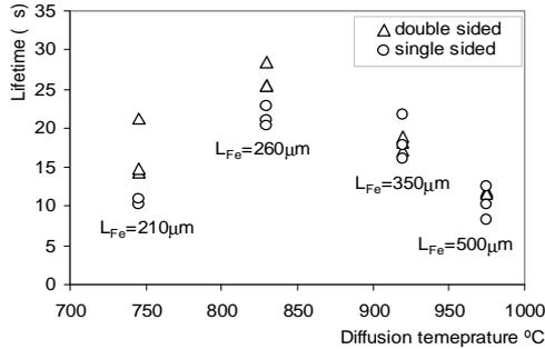
**Fig. 6** Minority carrier lifetime after single-sided versus double-sided emitter diffusion (column A<sub>1</sub>) at different temperatures.
