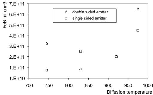
**Fig. 7** Dissolved FeB concentration in wafers from column A after single-sided versus double-sided emitter diffusion (column A<sub>1</sub>) at different temperatures.
