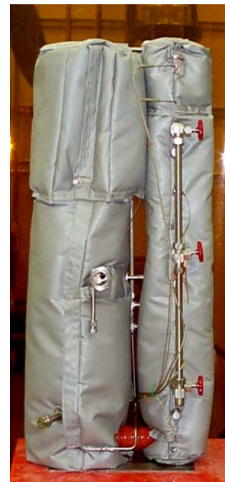
Figure 6 Micro-CHP PEM system with stack, humidifiers and inverter, control system.
