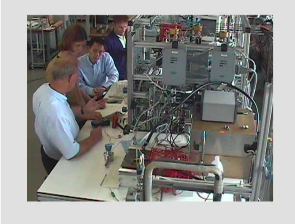
Figure 6 Micro-CHP PEM system with stack, humidifiers and inverter, control system.
