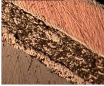
Figure 1b: Microscopic picture showing silver plated copper tab glued on silver plated silicon solar cell (upper right to lower left). The silver particles in the adhesive are clearly distinguishable in the picture.
