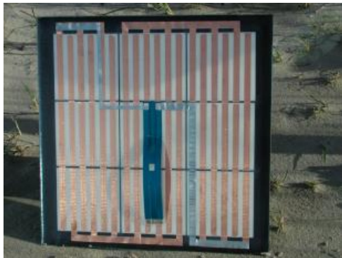
Figure 8: Busbarless EWT mini module. Active cell area is increased due to omission of the busbars compared to standard EWT cells. Current collection function of the busbars is taken over by rear-side interconnection foil.
