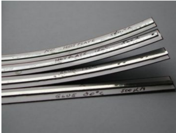
Figure 4: Bending due to stress of 300µm thick silicon strips with 2mm wide tabs. From back to front: soldering at 400°C on cold surface, soldering on 160°C hotplate, conductive adhesive cured at 160°C, conductive adhesive cured at 80°C.
