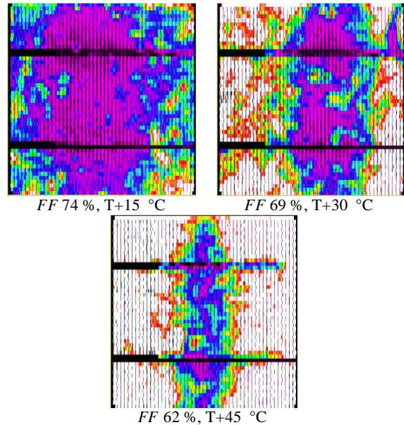
Figure 4: Corescans on cells fired at different set temperatures. Lighter areas have higher potential and thus higher contact resistance.
