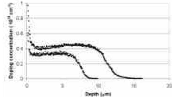
Figure 5: BSF at cell edge (upper curve) is about twice as deep as the BSF at the center of the cell.
