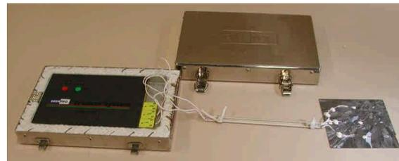
Figure 1: Data logger placed in opened thermal barrier with thermocouples attached to a wafer.
